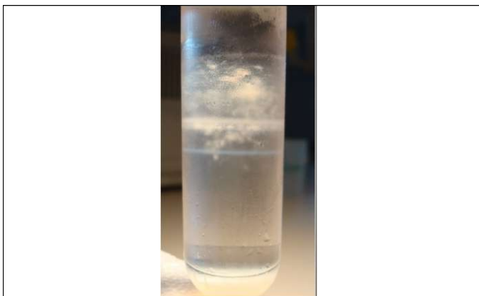
Fig. 3. White translucent band containing DWV particles after CsCl density gradient centrifugation.
