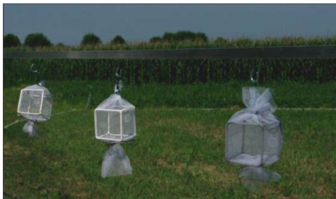
Fig. 2. Cages employed to expose bees to seed drill emissions and to evaluate survival after exposure.
