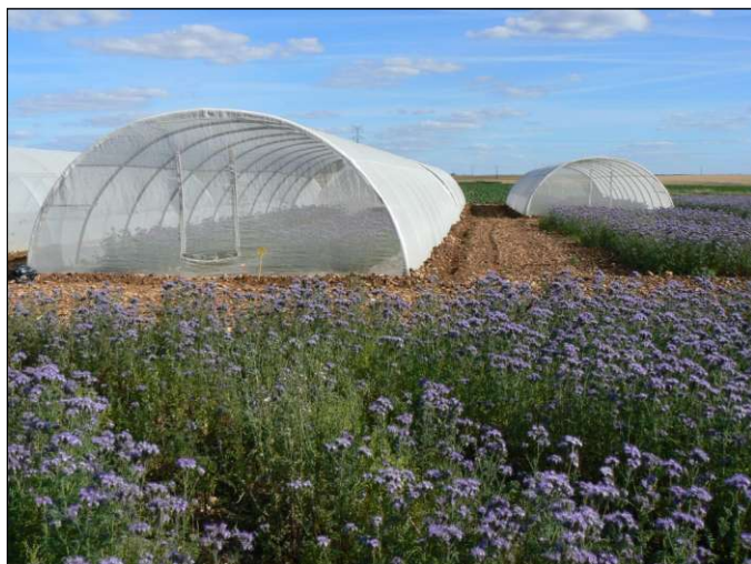
Fig. 7. Example of a tunnel used for semi-field toxicity tests.
