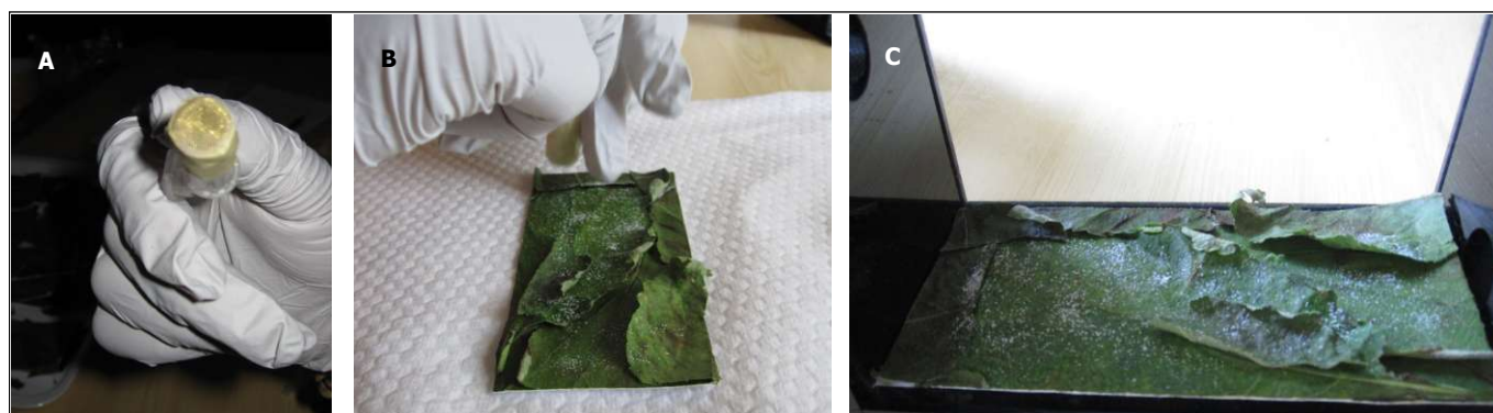
Fig. 1A. Small sieve obtained from a modified Eppendorf tube (the bottom is removed from the tube and replaced with screen mesh); B. Dust application on the apple leaves; C. Leaves placed in the bottom of the hoarding cage.
