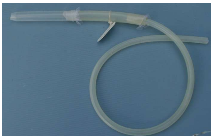
Fig. 4. Insect vacuum (aspirator) used to capture the bees. The two mesh diaphragms safely prevent the bee from being sucked into the mouth of the operator.
