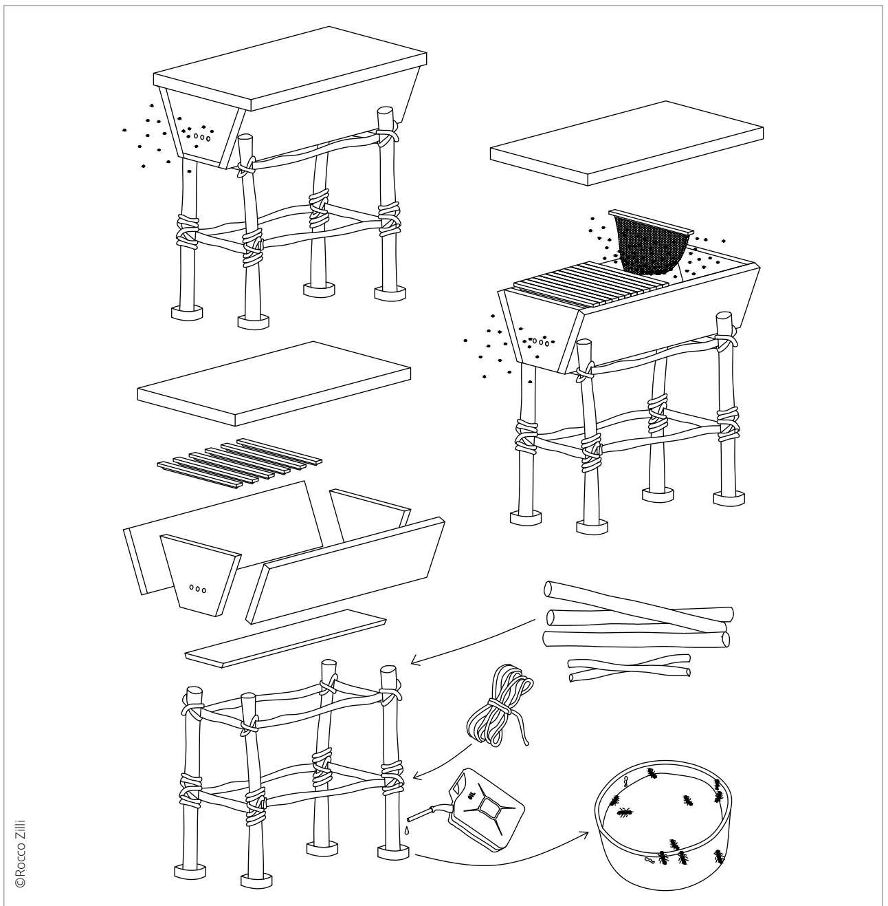
Figure 5: A top bar hive installed on a hive stand
