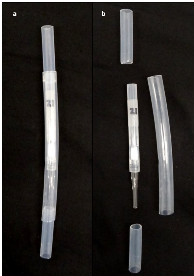
Fig. 2. (a) Assembled and (b) unassembled views of a SuperQ adsorbent filter enclosed in a protective Teflon tube jacket made of interlocking sections of tube.
