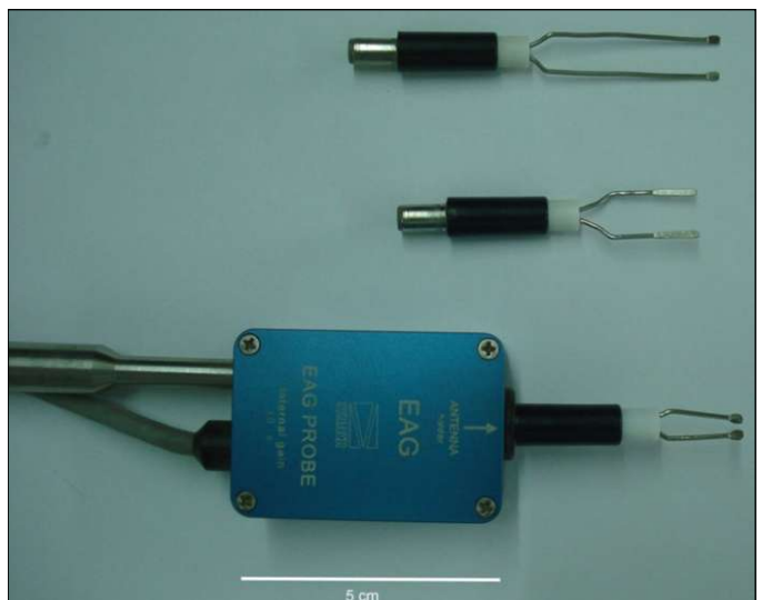
Fig. 5b. Gel electrodes and probe. Electrodes vary in their sizes fitting both large and small antennae or chemosensory organs.
