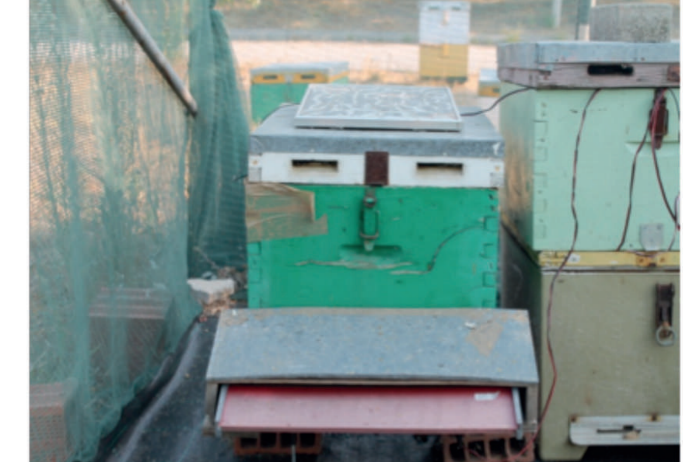
Fig. 4. The bee counter attached on the entrance of the colony. The solar panel on top of the colony was charging the battery used for the micro-processor.
